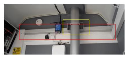
This fitting solution will assist all installations of masts within the Mercedes Sprinter High COMPOSITE Roof vehicle model. Designed by Pressfab EVO Limited and manufactured by Pressfab Engineering Limited. The kit is in two parts, as highlighted, and excludes the base and roof top parts, although we could discuss these.
